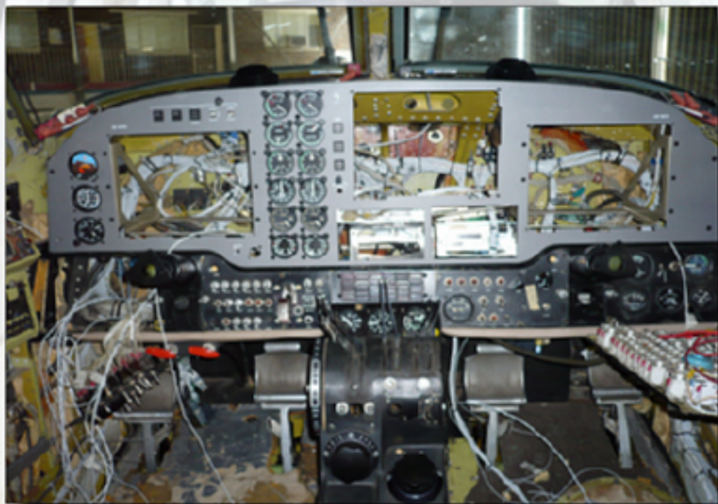
Fitting engine and standby gauges
